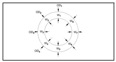
Figure 3-6: Measuring the OD and Pipe Wall Thickness
